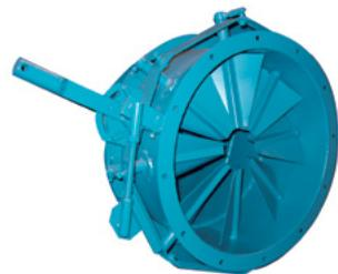
Two types of inlet vanes are offered, depending on fan size. Inlet vanes for sizes 122, 135, and 150 are external type, bolted to the fan inlet flange. Inlet vanes for sizes 165 and larger are supplied as nested type, with the inlet vane blades nested within the inlet cone and all linkages internal to the fan. (Nested style inlet vanes shown.)
